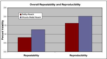
Data taken from the ASTM Test Monitoring Center (TMC) Round Robin study are shown in the adjacent graphs. The Selby-Noack has very good correlation to the Wood's Metal Noack with better overall precision.
