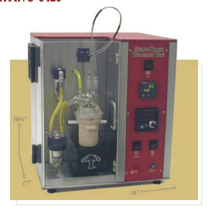
The original Noack evaporation loss test has been known and used in the industry since the 1930's. It uses a toxic mixture of compounds known as Wood's Metal for sample heating. In the mid-1990's, Mr. Selby and his coworkers at Savant, Inc. eliminated the need for Wood's Metal by devising a noble-metal heater approach. When thorough developmental work on the Selby-Noack was completed in 1997, Tannas began marketing the first non-Wood's Metal Noack tester.
